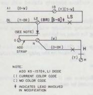
Fig. 1-Station Busy Lamp (Without | Hold Feature)
