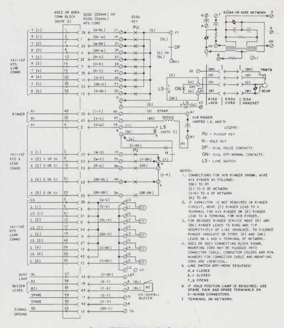
Fig. 4-\$564HLM Telephone Set, Connections
