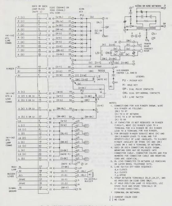
Fig. 3-\$564HK (MD) and 564HL Telephone Set, Connections
