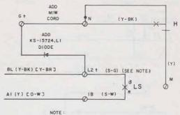
(S-G) LINE SWITCH LEAD INVOLVED IN MODIFICATION WAS ORIGINALLY CONNECTED TO TERMINAL N.
