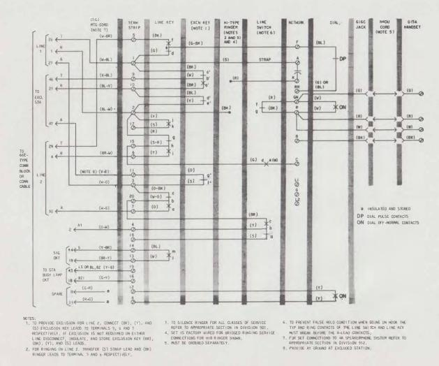
Fig. 2—558FM Telephone Set Connections Wired for 2-Line Pickup With Exclusion on Line 1, Signaling, and Speakerphone (Factory Wired)
