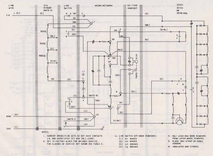
Fig. 5-\$25548 Telephone Set E/W 4228K Network, Connections (Foctory-Wired)
