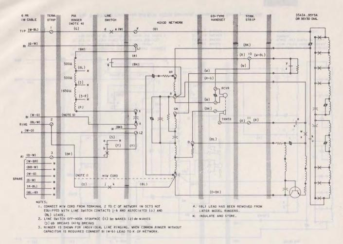
Fig. 6—\$25548 Telephone Set E/W 4010D Network, Connections for 1A1 or 1A2 Key Telephone System\$
