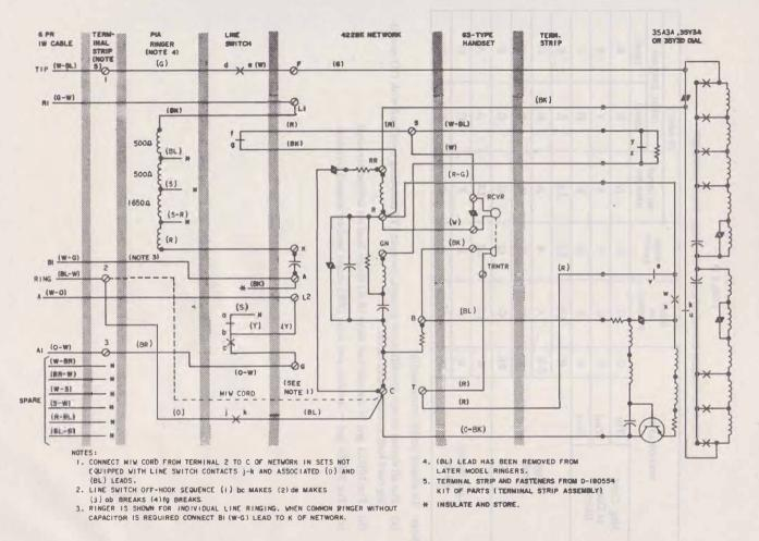
Fig. 7—\$2554B Telephone Set E/W 4228K Network, Connections for 1A1 or 1A2 Key Telephone Systems
