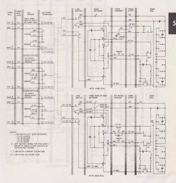
Fig. 2-1500D Telephone Set, Connections
