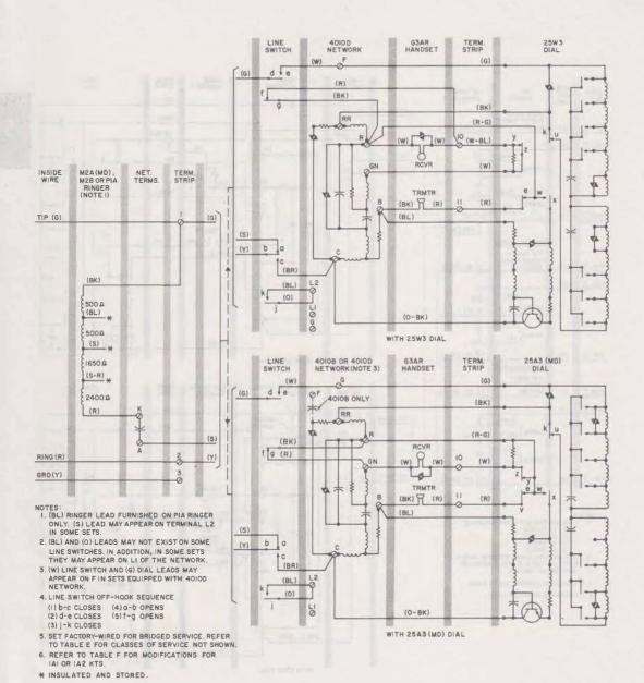
Fig. 3-1554B(MD) Telephone Set, Connections
