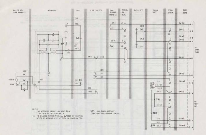
Fig. 5—513B (MD) Telephone Set, Connections
