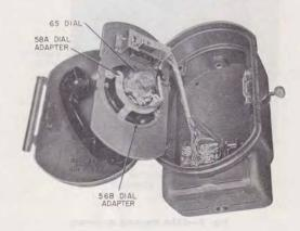
Fig. 2—525B (MD) Telephone Set (Dial), Inner Door Open
