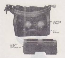
Fig. 8—525 (MD)-Type Telepone Set, Cover Assembly
