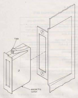
Fig. 4—♦Partial View of 526A Housing Assembly, Installation of Magnetic Catch€
