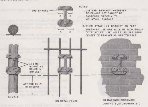
Fig. 7—29D Bracket Mounted on Various Surfaces
