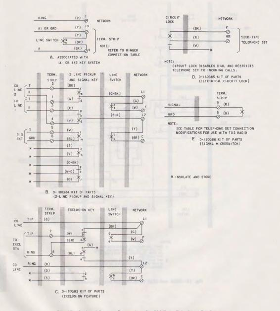
Fig. 17—Optional Feature Connections for 526-Type Telephone Set Bases
