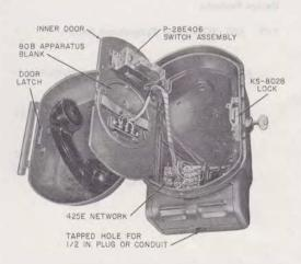
Fig. 1—525A (MD) Telephone Set (Manual), Inner Door Open
