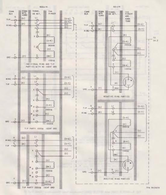
Fig. 5—500J/K (MD) and 501J/K (MD) Telephone Sets, Connections (Sheet 1 of 2)
