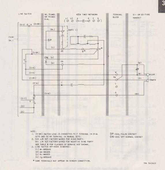
Fig. 5—500J/K (MD) and 501J/K (MD) Telephone Sets, Connections (Sheet 2 of 2)
