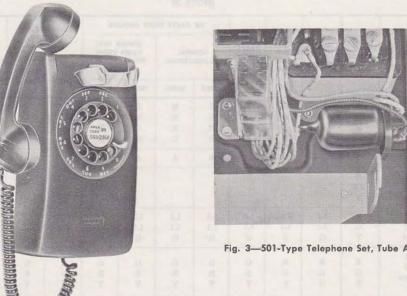
Fig. 3-501-Type Telephone Set, Tube Assembly
