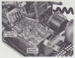
Fig. 12—\$819040528 (P-90D052) Guard Assembly, Installed
