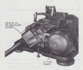
Fig. 8—Location of KS-8109L2 Buzzer
