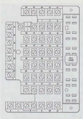
Fig. 3—Terminal Board for the 636B Key
