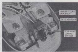
AINSTALLING 282B ADAPTER ON EXISTING HANDSET CORD JACK
