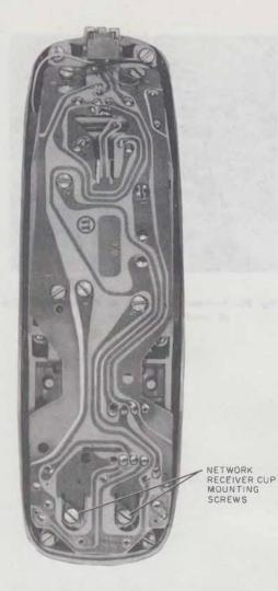
Fig. 15—2220C Hand Telephone Set Showing Location of Network Mounting Screws
