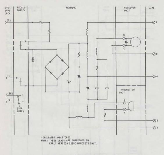
Fig. 28—Schematic of 2220C Hand Telephone Set
