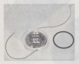
Fig. 12—Receiver Unit Installed in Coil Assembly
