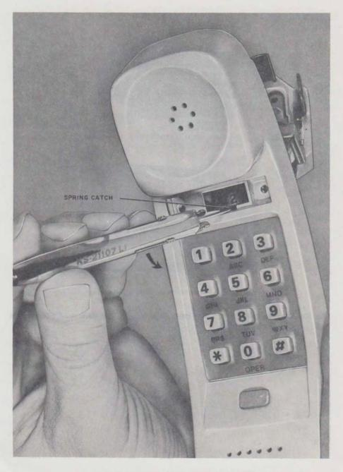
Fig. 21—Releasing Spring Catch on 315-Type Amplifier
