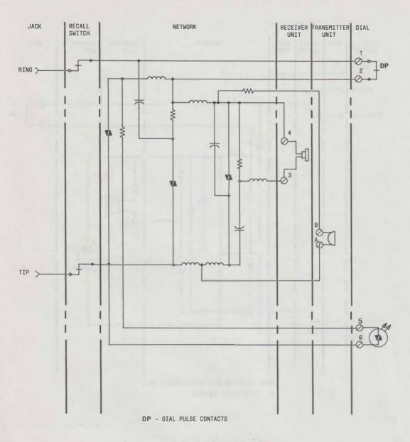
Fig. 24—Schematic of 220C Hand Telephone Set
