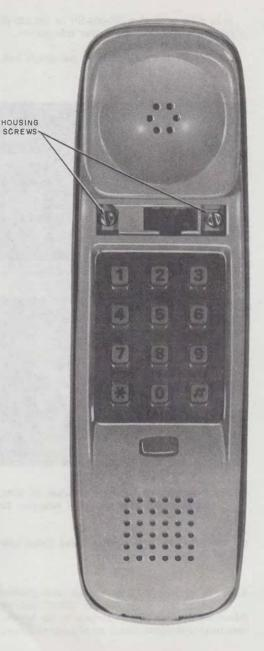
Fig. 6—Location of Housing Screws
