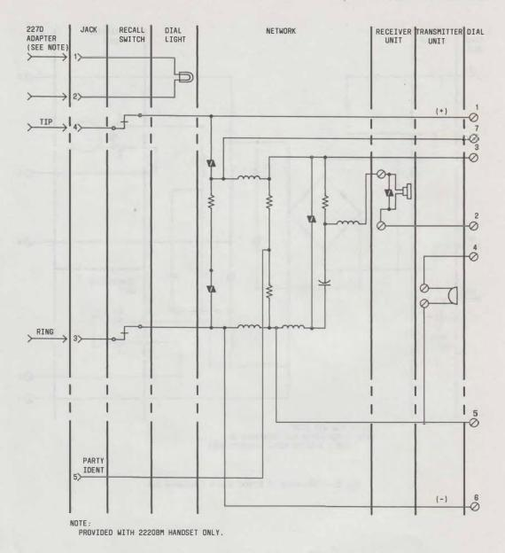
Fig. 27—Schematic of 2220B (MD) and 2220BM Hand Telephone Set
