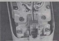
B. 282B ADAPTER INSTALLED ON HANDSET CORD JACK
