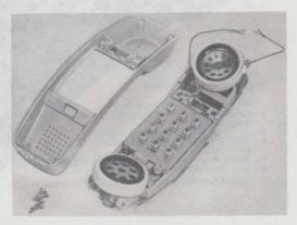
Fig. 14—Field Coil Installed in Receiver Cup of Chassis Assembly
