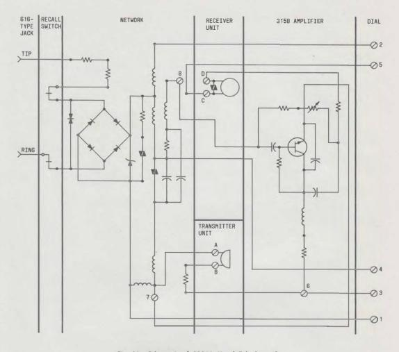
Fig. 29—Schematic of 2226A Hand Telephone Set
