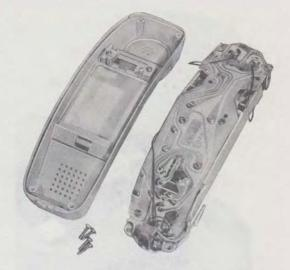
Fig. 16—Terminating Field Coil Leads to Receiver Cup Mounting Screws
