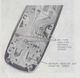
Fig. 19—Location of Mounting Screws Used to Connect Amplifier in Hand Telephone Set
