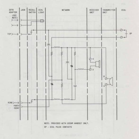
Fig. 23—Schematic of 220A (MD) and 220AM Hand Telephone Set
