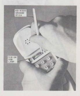
Fig. 17—Removing Dial Lamp from 2220BM Hand Telephone Set
