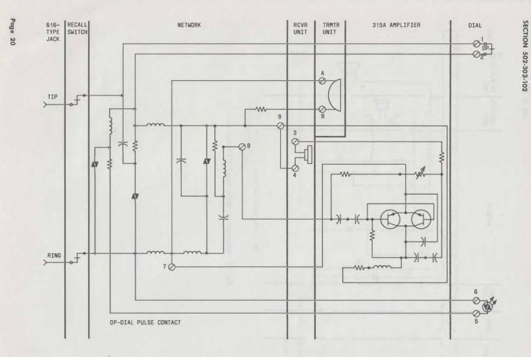
Fig. 26—Schematic of 226A Hand Telephone Set
