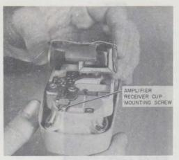
Fig. 20—Fastening Amplifier to Receiver Unit Cup of Hand Telephone Set
