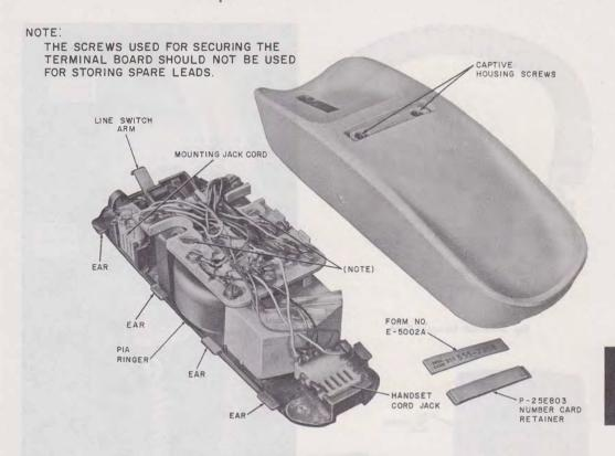
Fig. 4—Interior of AD1 Telephone Base
