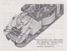
Fig. 8—P-90D231 Polarity Guard Assembly, Installed
