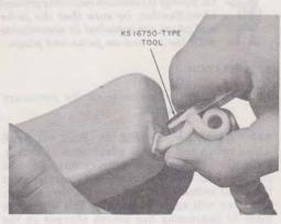
Fig. 15—Removing Handset Cord From the Hand Telephane Set
