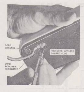
Fig. 16—Removing Mounting Cord From AD1 Telephone Base
