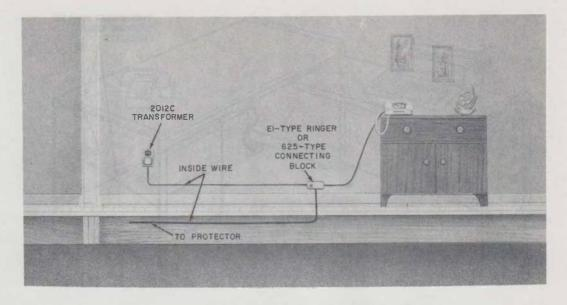
Fig. 4—Typical Installation of 700-Type Telephone Set
