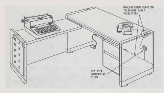
Fig. 6—Desk With Built-in Wire Channel and Desk Top Opening for Telephone Wire
