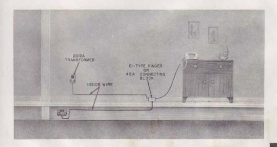
Fig. 4—Typical Installation of 700-Type Telephone Set
