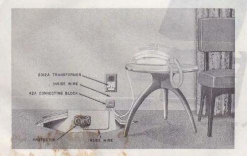
Fig. 1—Typical Installation of AD1 Telephone Base With 220A Hand Telephone Set
