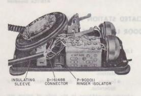
Fig. 2—Ringer Isolator in 500-Type Telephone Set
