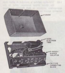
Fig. 3-Ringer Isolator in 74-Type Connecting Block
