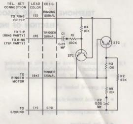
Fig. 4—P-90D011 Ringer Isolator—Schematic
