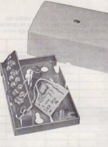
Fig. 7—10A Extender Mounted in a 74C Connecting Block
