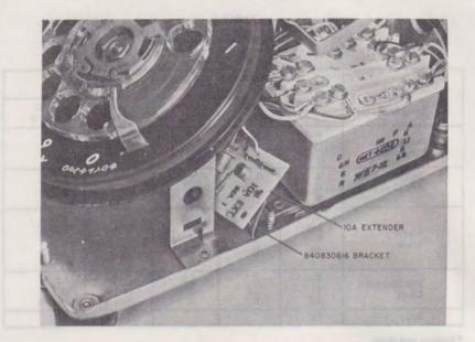
Fig. 5—10A Extender Installed in a 500-Type Telephone Set
