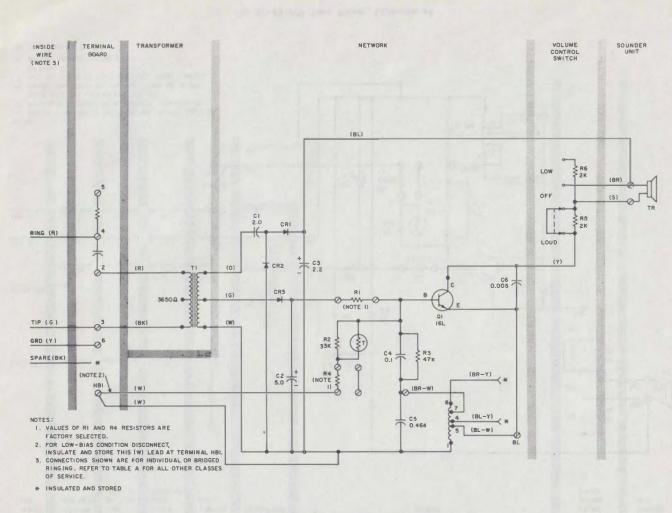
Fig. 5-SIA (MD) Tone Ringer, Connections
