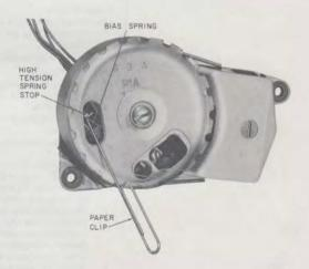
Fig. 6—Positioning Bias Spring
