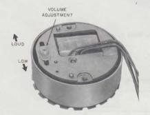
Fig. 4—P-Type Ringer (Bottom View)
