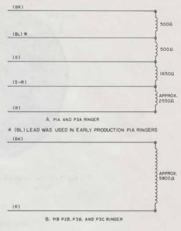
Fig. 5—PP-Type Ringer—Schematic
