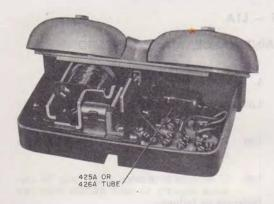
Fig. 3 - L1A Ringer with 425A or 426A Tube
