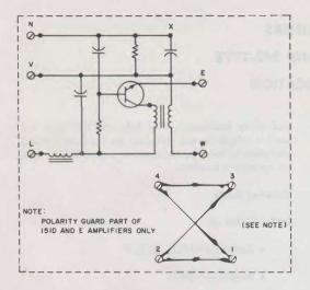
Fig. 1—151-Type Amplifier and Polarity Guard,
