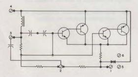
Fig. 3-4241B Amplifier Schematic
