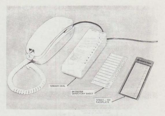
Fig. 4—1200AR1 Dial With Faceplate and Directory Sheet Removed
