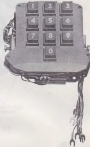
Fig. 1—10-Button 25-Type Nonconvertible Dial, Front View
