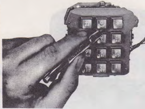
Fig. 8—Removing Special Service Button
