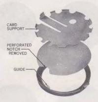
Fig. 7—Method of Placing Number Card in Holder
