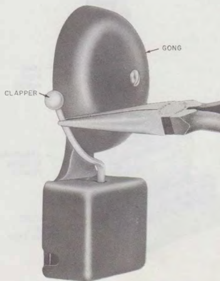
Fig. 19—Adjusting Clapper Movement
