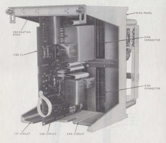
Fig. 4—102B Interconnecting Unit Mounted in 615A Panel
