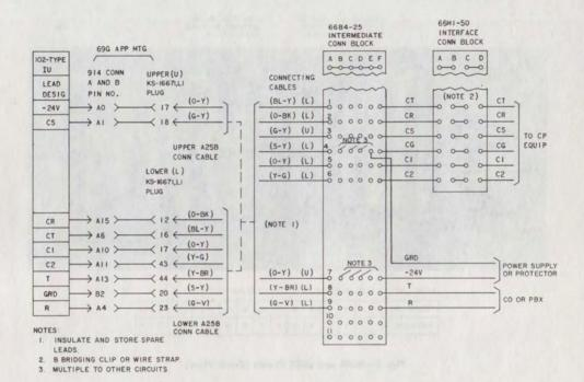
Fig. 5—Connection Diagram for 69G Apparatus Mounting
