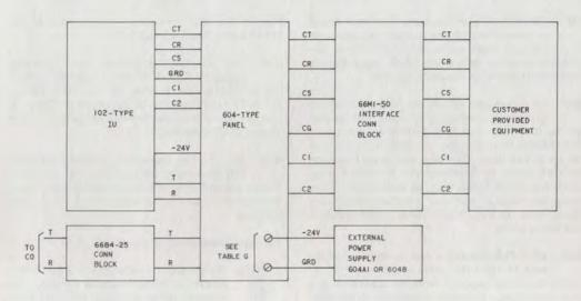
Fig. 7—Block Diagram—102-Type Interconnecting Unit With 604-Type Panel
