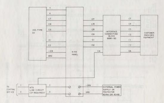
Fig. 8—Block Diagram—102-Type Interconnecting Unit With 615A-Type Panel
