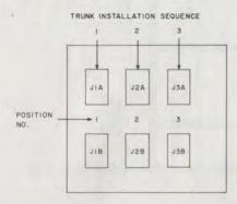
Fig. 11—Connector and Trunk Arrangement in 615A
