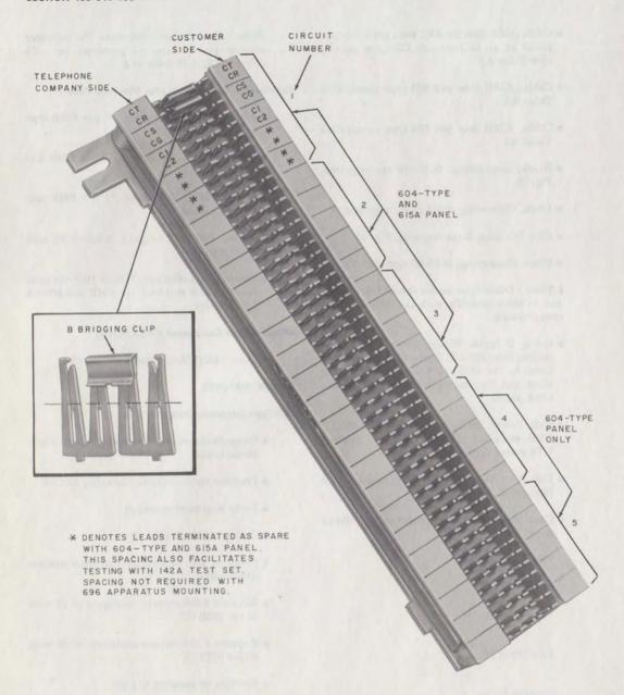
Fig. 2—66M1-50 Interface Connecting Block
