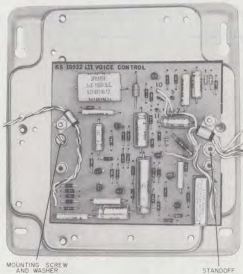
Fig. 9—KS-19522, List 11 Voice Control, Mounted on Baseplate
