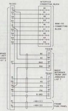
Fig. 5—Connections Between Applique Unit, Interface Connecting Block, Basic Interface Trunk Unit, and Frame Fuse Panel to Convert Dial Pulse Digits to CP Equipment for 2- out of 7-Lead dc Signals
