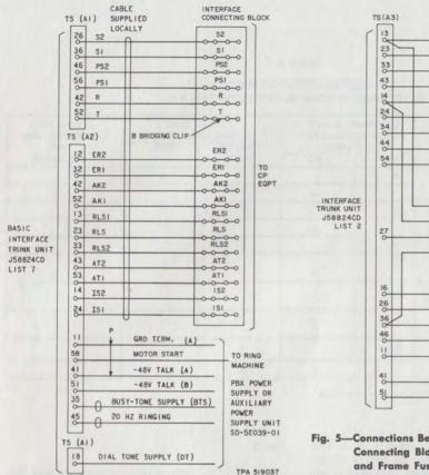
Fig. 4—Connections Between Basic Interface Trunk Unit, Interface Connecting Block, Frame Fuse Panel, Busy-Tone Supply and 20-Cycle Ringing Supply for Rotary Dial Pulsing or TOUCH-TONE Signaling
