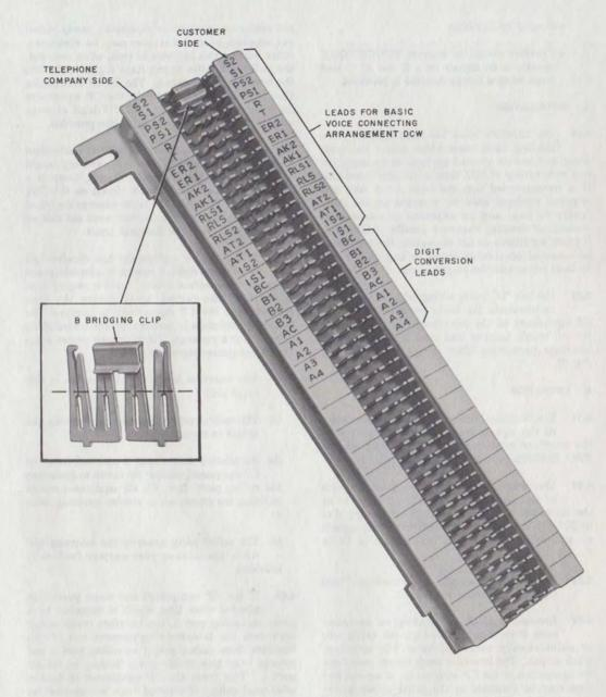
Fig. 2—Typical Interface Connecting Block
