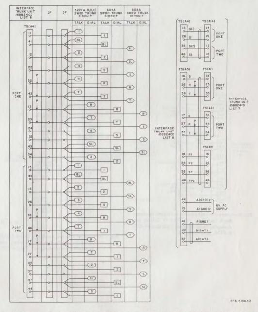
Fig. 9—Connections Between 552A, B, D, E, 605A, 608A Switchboard Talk and Dial Jack Circuits, Applique Unit, Basic Interface Trunk Unit, Frame Fuse Panel, and 6-Volt Supply to Provide Calling Party Access From Switchboard
