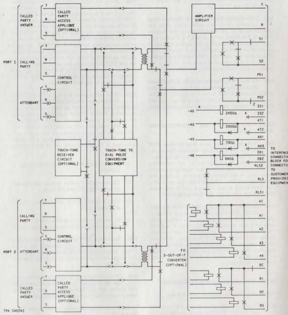
Fig. 3—Simplified Schematic—Voice Connecting Arrangement DCW
