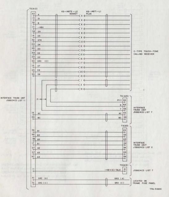
Fig. 8—Connections Between Applique Units, C-Type TOUCH-TONE Receiver, Basic Interface Trunk Unit, and Frame Fuse Panel to Convert TOUCH-TONE Signals to dc Signals on a 2- out of 7-Lead Basis
