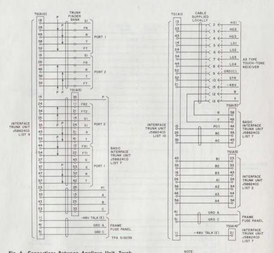
Fig. 6—Connections Between Applique Unit, Trunk Finder Bank Circuit, Basic Interface Unit, and Frame Fuse Panel to Convert TOUCH-TONE Signals to Dial Pulses
