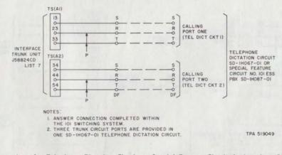
Fig. 16—Connections for Telephone Dictation Circuit or Special Feature Circuit Assigned to Calling Ports of Interface Trunk Circuit—No. 101 ESS
