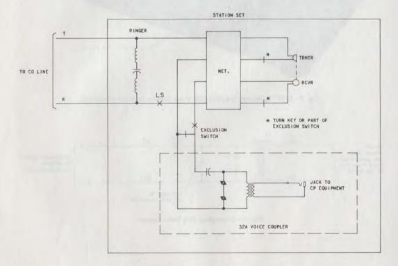
Fig. 5—Schematic-Voice Connecting Arrangement QKP
