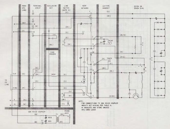
Fig. 7—2502B Telephone Set—Modified for Use With 32A Voice Coupler
