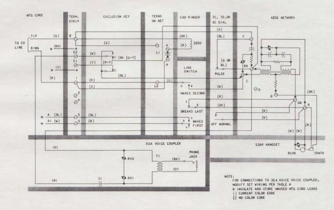
Fig. 6-502B Telephone Set-Modified for Use With 32A Voice Coupler
