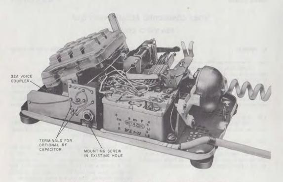
Fig. 2-32A Voice Coupler Mounted in 2511F Telephone Set (Cover Removed)
