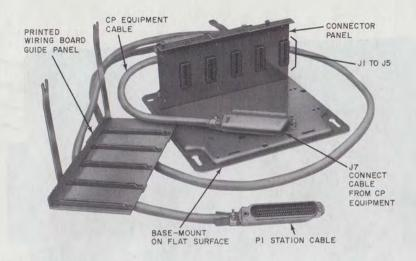
Fig. 2—KS-20893,List 11 Interconnecting Service Unit, Unequipped (Cover Removed)
