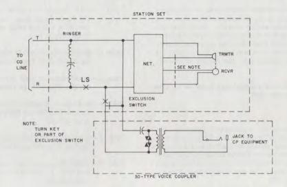
Fig. 3—♦Schematic—Voice Connecting Arrangements QKT and QKTBT
