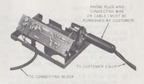
Fig. 2-30-Type Voice Coupler, Cover Removed
