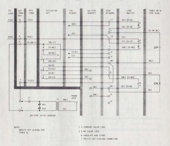
Fig. 4—Typical Telephone Set—Modified for Use With 30-Type Voice Coupler Using Exclusion Key to Automatically Disable Transmitter and Receiver
