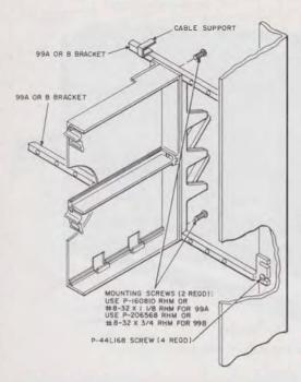
Fig. 7—69-Type Apparatus Mounting on a 99A (MD) ar 99B Bracket
