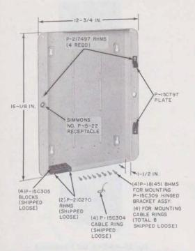
Fig. 21—177A Aluminum Backboard Assembly (MD)
