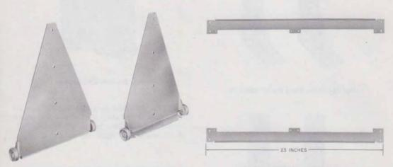
Fig. 39—Bracket Assembly Per ED-69366-50, Group 2
