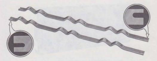
Fig. 42—Bent Mounting Bars Per ED-69143-70
