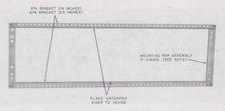
Fig. 41—67-Type Brackets for Mounting Panel Type 200-Series Key Telephone Units
