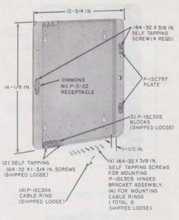
Fig. 22—177A Fiber Glass Backboard Assembly
