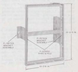
Fig. 4—31B Apparatus Mounting
