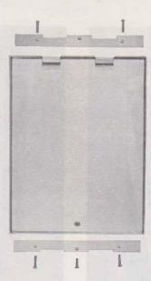
Fig. 17—107B Apparatus Blank and Mounting Hardware
