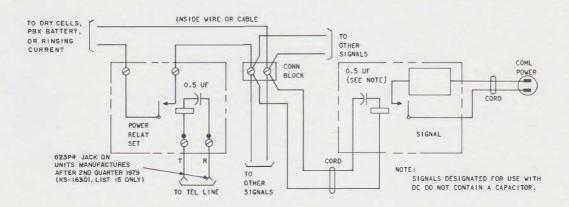
Fig. 22—Multiple Signal Connections
