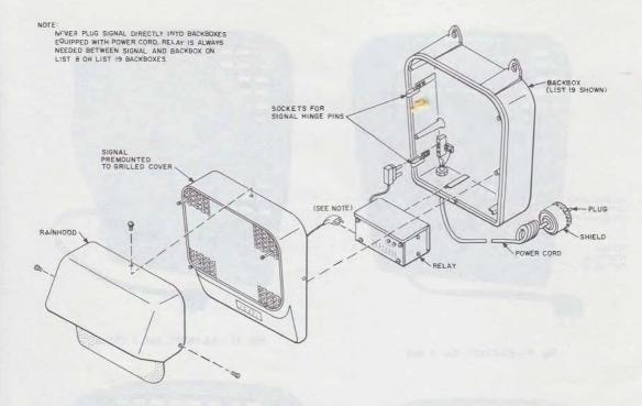
Fig. 7—KS-16301-Type Signal—Exploded Assembly
