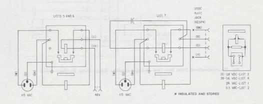
Fig. 24—Connections for KS-22001 Chimes
