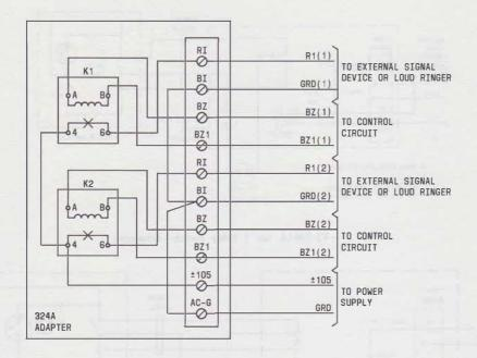
Fig. 29—Connections for 324A Adapter
