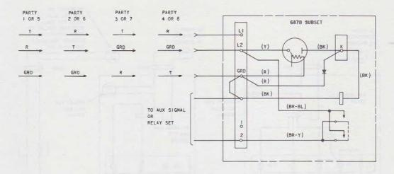
Fig. 25—Connections for Auxiliary Signals on Party Line Using CO Ringing Power
