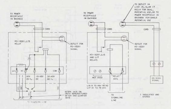
Fig. 23-KS-16301 Signal Connections
