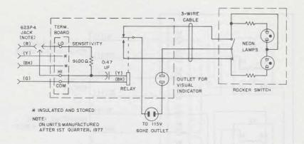
Fig. 27—KS-20614, List 1 Relay Switch—Schematic
