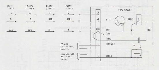
Fig. 26—Connections Party Line Low Voltage Auxiliary Signal Using Auxiliary Power
