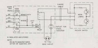
Fig. 31—KS-20614, List 1 Relay Switch—Schematic
