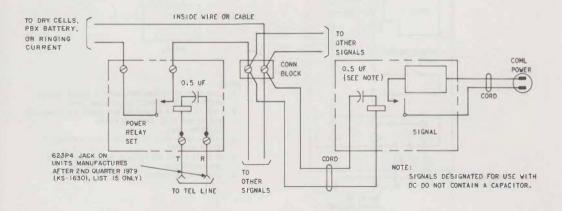
Fig. 25—Multiple Signal Connections
