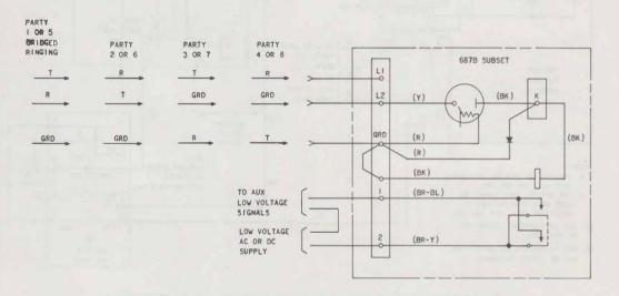
Fig. 29—Connections for Noncontinuous Low Voltage Auxiliary Signal
