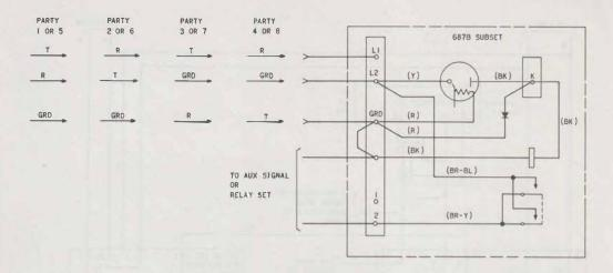
Fig. 28—Connections for Auxiliary Signals on Party Line
