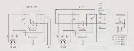
Fig. 33—Connections for KS-22001 Chimes
