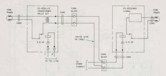
Fig. 26—KS-8233, List 2 Transformer Relay Connections
