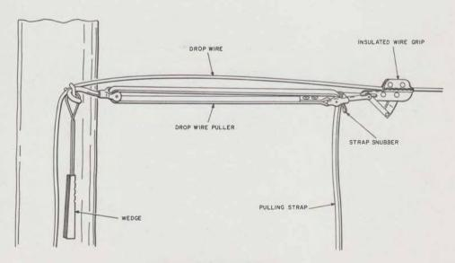
Fig. 3—Tensioning Drop Wire
