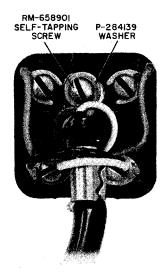
Fig. 13—D4BP Cord Terminated on 283B Plug
