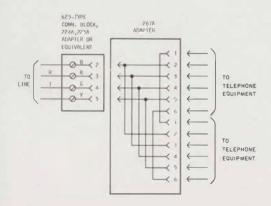
Fig. 15—Schematic Diagram, 267A Adapter
