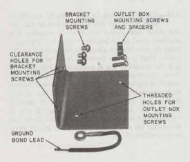
Fig. 61—B Mounting Bracket (for Mounting B Outlet Box)
