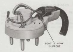
Fig. 49—Early Model D3BU Cord Connected to 505A
