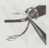
Fig. 43—Bending S Hook
