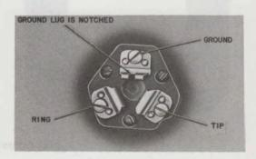
Fig. 22—Connections for KS-8420 and KS-8421 Jacks (MD)
