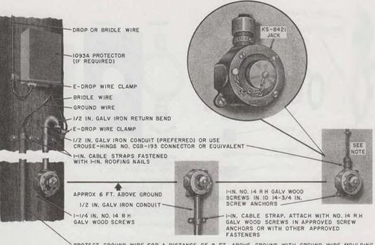
PROTECT GROUND WIRE FOR A DISTANCE OF 8 FT. ABOVE GROUND WITH GROUND WIRE MOULDING. PLACE STRAPS APPROX 4 FT. APART. IF POLE IS CROOKED, PLACE SUFFICIENT STRAPS TO MAKE MOULDING CONFORM TO CONTOUR OF POLE.
