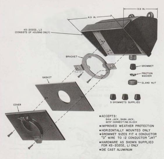
Fig. 29—Assembly of KS-20202, List 1 and 2 Waterproof Housing
