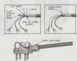
Fig. 51—Connecting Current Model D3BU or D4BP Cord to Early Model 505A Plug
