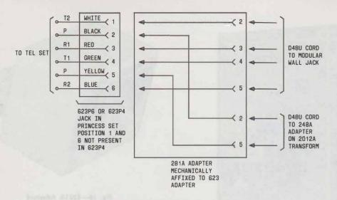
Fig. 17— Schematic Diagram, 281A Adapter
