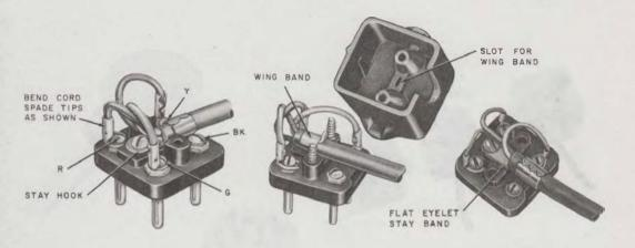
Fig. 41—Terminating Cords Equipped With a Stay Hook, Wing Band, or Flat Eyelet Stay Band on a 283B (MD) Plug
