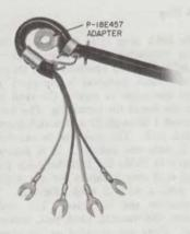
Fig. 42—Early Model D4BP Cord and Adapter
