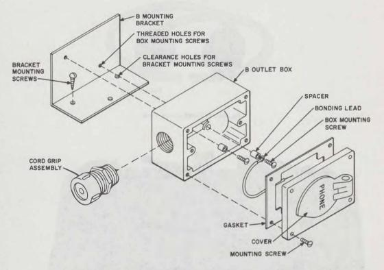
Fig. 63—Assembly of B Weatherproof Male Jack to B Outlet Box and B Mounting Bracket
