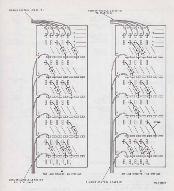
Fig. 8—Wiring Arrangement and Diode Orientation
