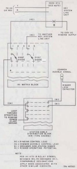
▶ Fig. 7—Block Schematic Layout ♠
