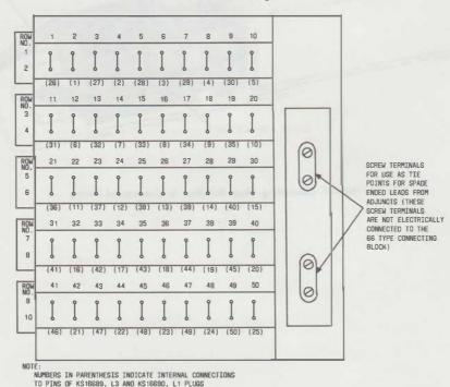
Fig. 7—♦Numbering and Wiring Plan for 66E8-25 Connecting Block♦
