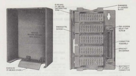
Fig. 1-66E3-25 Connecting Block
