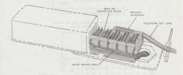
Fig. 5-66E4-25 Connecting Block Installed in Commercial Fitting
