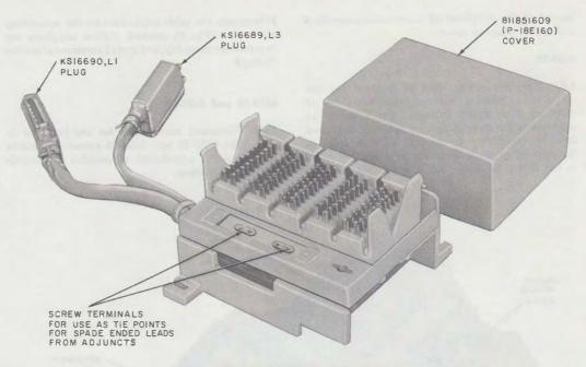
Fig. 3-\$66E8-25 Connecting Block\$
