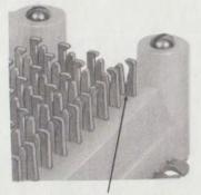
THESE TERMINAL BEAMS CANNOT BE CORRECTED AND THE TERMINAL MUST NOT BE USED
