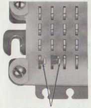
BENT TERMINAL BEAMS
