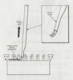
Fig. 4-Removing Conductor With 724A Tool
