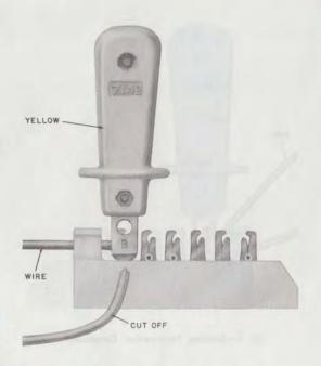
Fig. 10-Ended Termination Completed
