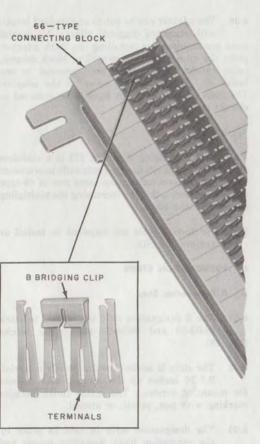
Fig. 17—B Bridging Clip, Installation Detail
