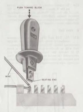
Fig. 5—Preparation for Looping Termination
