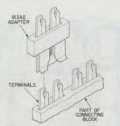
Fig. 13-183A2 Adapter, Installation Detail
