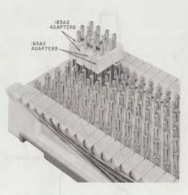
Fig. 14—Typical Installation of 183A2 Adapters on 66B-Type Connecting Block
