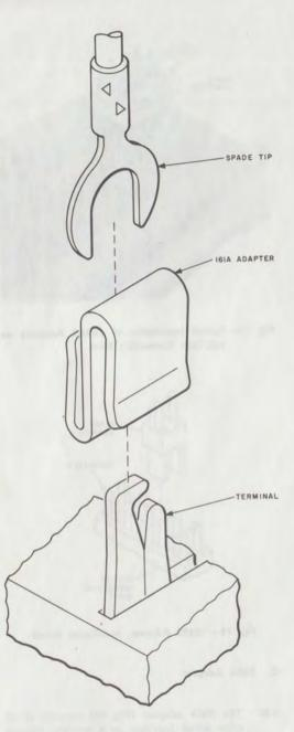
Fig. 11-161A Adapter, Installation Detail
