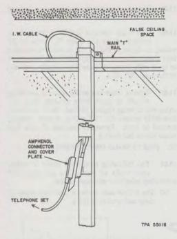
Fig. 11—Utility Column Installation
