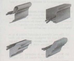
Fig. 7—Wiring in Picture Moldings
