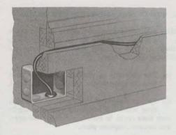
Fig. 5—Wiring From Conduit to Baseboards
