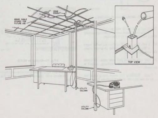
Fig. 10-Wiring Method With Utility Columns 4
