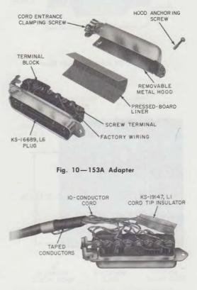
Fig. 11-10-Conductor Cord in 153-Type Adapter
