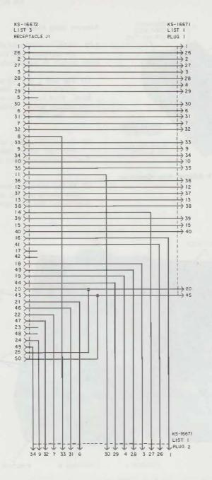
Fig. 21—KS-19252, List 5 3-Way Bridging Adapter Schematic
