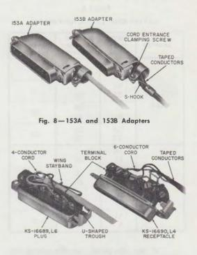
Fig. 9—153A and 153B Adapters, Hood Removed
