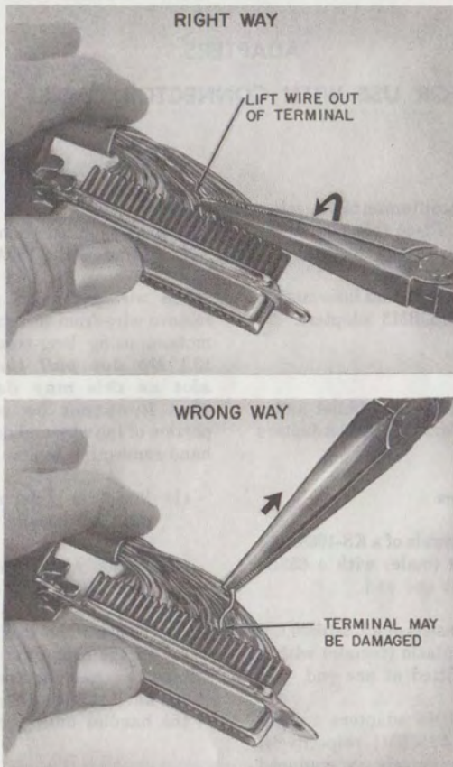
Fig. 13.1—Removing Terminated Wire
