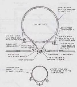
Fig. 8—Attachment to Type 188 Sign Bracket
