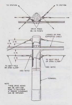
Fig. 2—Terminal Mounted on Cable Side of Pole
