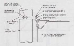
Fig. 7—Attachment to Type 170 Sign Bracket
