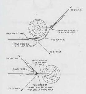
Fig. 5—Distributing Wires From Pole Other Than Terminal
