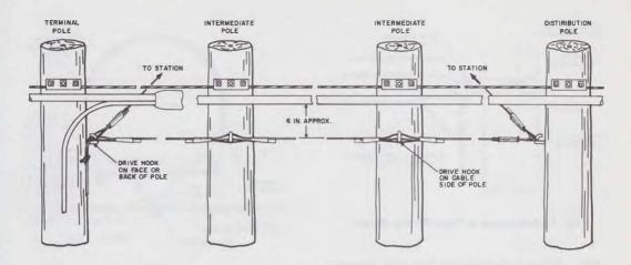
Fig. 4—Drop Wire Run Along Lead Carrying Cable
