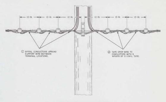
Fig. 14—Arrangement of Wire Terminals
