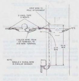
Fig. 13—Pole Attachment of Block and Rural Wire
