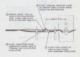
Fig. 10—Attaching 105A Wire Terminal
