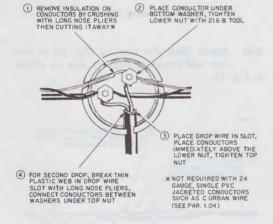
Fig. 12—Terminating Wire Leads
