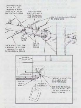
Fig. 1—Where Drop Wire is Distributed From Crossarms
