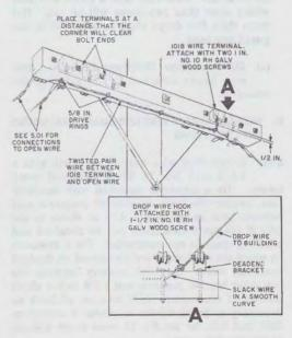
Fig. 3—Wiring Arrangement on DE Crossarms not Having Back Braces
