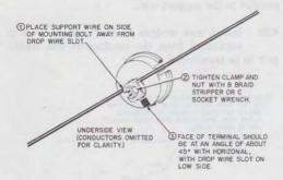
Fig. 11—Attaching Support Wire
