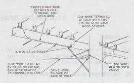
Fig. 2—Where Drop Wire is Distributed From a Pole
