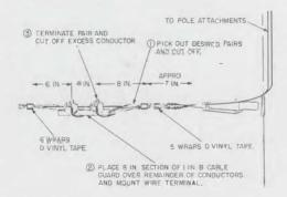
Fig. 15—Location of Wire Terminals at Dead-End
