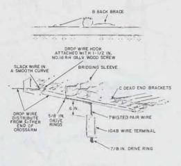
Fig. 4—For More Than Two Drops Use a 104B Wire
