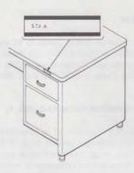
Fig. 5—Method of Marking New Telephone Locations on Presurvey Using Form E-5826
