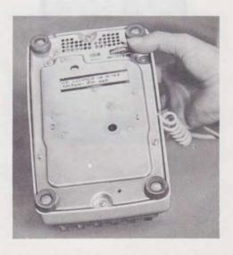
Fig. 2—Marking Cable Location Using Form E-5826
