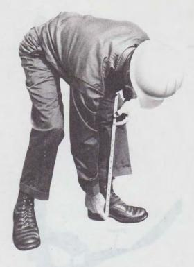
Fig. 8—Measuring for Climber Length
