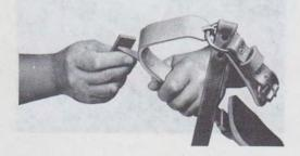
Fig. 17—PRemoving Burrs From Top Cutting Edge ◆
