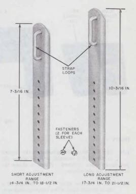
Fig. 3— Sleeves for Adjustable Climbers
