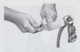
Fig. 18—▶Removing Burrs From Bottom Cutting Edge ♦
