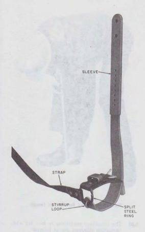
Fig. 5-Foot Straps Attached to Climbers
