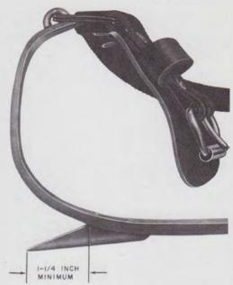
Fig. 21—Gaff Sharpened to Minimum Length
